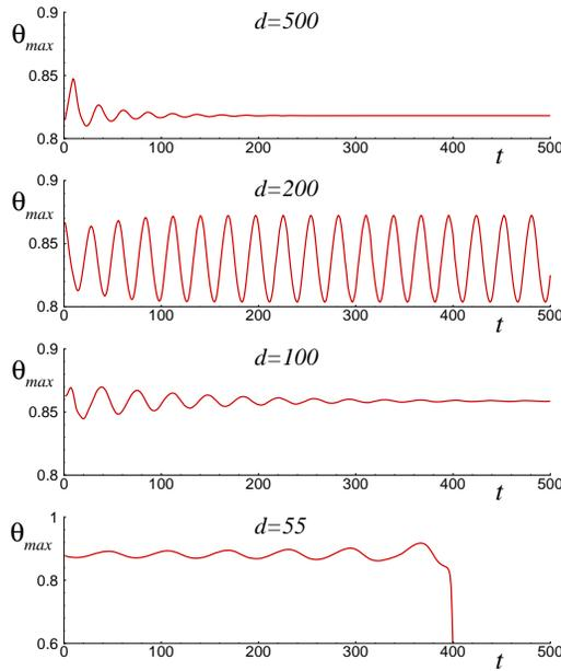
Figure 4: Time history of the maximum temperature in the domain for  $Le = 1$ ,  $Re = 120$  and various  $d$ . The case  $d = 55$  represents the oscillatory behavior with an increasing amplitude and, finally, the flame extinction; the case  $d = 200$  exhibits the oscillatory behavior.
