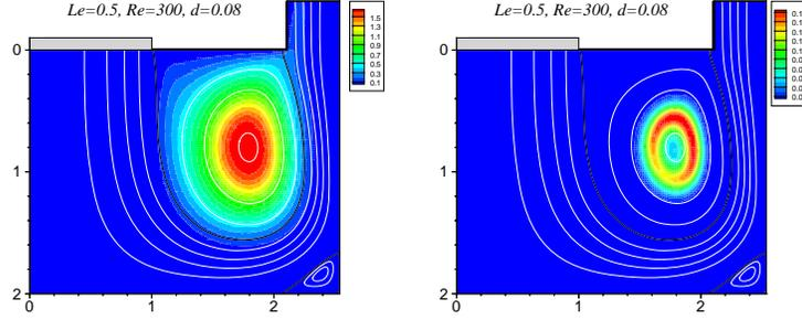
Figure 5: Temperature (a), reaction rate (b) contours and the isolines of the stream function computed for  $Le = 0.5$ ,  $Re = 300$  and  $d = 0.08$ . The isolines of  $\psi$  at same intervals as in Figs. and 2.
