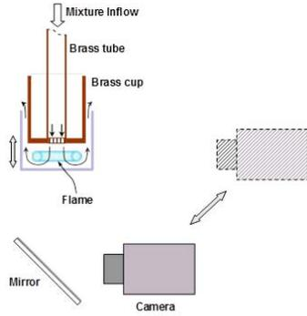
Figure 8: Schematic of the experimental setup.
