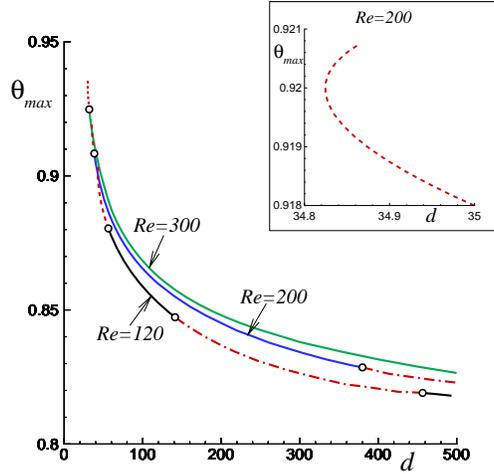
Figure 3: The steady-state maximum temperature as a function of  $d$  for several Reynolds number calculated for  $Le = 1$ : solid segments - stable steady states; dashed segments - unstable steady states (flame extinction); dashed-dotted segments - oscillatory behavior. Open circles indicate the marginal states.
