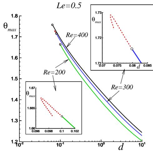
Figure 6: The steady-state maximum temperature as a function of  $d$  for several Reynolds numbers calculated for  $Le = 0.5$ ;  $\theta = 1$  corresponds to adiabatic flame temperature; solid segments - stable steady states; dashed segments - unstable steady states (flame extinction).
