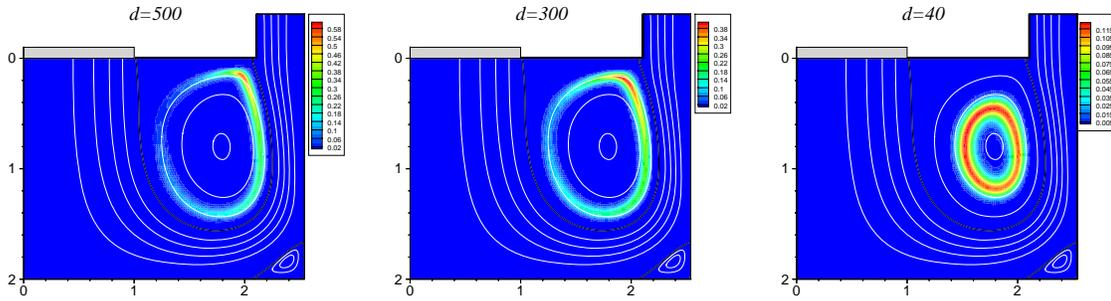
Figure 2: Reaction rate contours (color plot) and the isolines of the stream function computed for several values of  $d$  and  $Re = 300$ ,  $Le = 1$ . The isolines of  $\psi$  are at same intervals as in Fig. .
