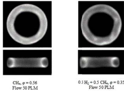
Figure 9: Bottom and side views of toroidal flames of methane-air (left) and hydrogen-methane-air (right) mixtures.
