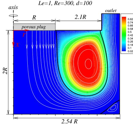
Figure 1: Sketch of the numerical problem, coordinate system, the temperature field (color plot); the isolines of the stream function computed with  $Re = 300$ ,  $Le = 1$  and  $d = 100$  are plotted with white lines; the thick black lines show the separation values  $\psi = 0$  and  $0.5$ ; the isolines inside the corner recirculation region at the corner  $\psi = -0.002$  and  $-0.004$ ; the isolines outside the corner recirculation region at interval of  $0.05$ .
